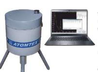
Matrix method allows measurement of volumetric (specific) activity for monitored radionuclides based on energy windows count rate.
